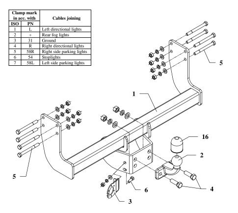
This towing hitch is designed to assembly in following cars: **MERCEDES SPRINTER5 ton, loading platform, double wheels** produced since 06.2006 to 05.2018, **VOLKSWAGEN CRAFTER 5 ton, loading platform, double wheels** produced since 04.2006, catalogue no. **D40** and is prepared to tow trailers max total weight up to **3500 kg** and max vertical mass **140 kg**.
