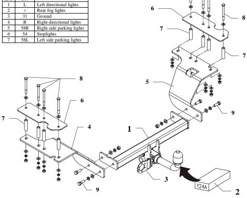
This towbar is designed to assembly in following cars: HONDA CR-V, 5 doors produced since 04.2002 till 01.2007, catalogue number Y24A and is prepared to tow trailers max total weight 1690 kg and max vertical mass 100 kg.
