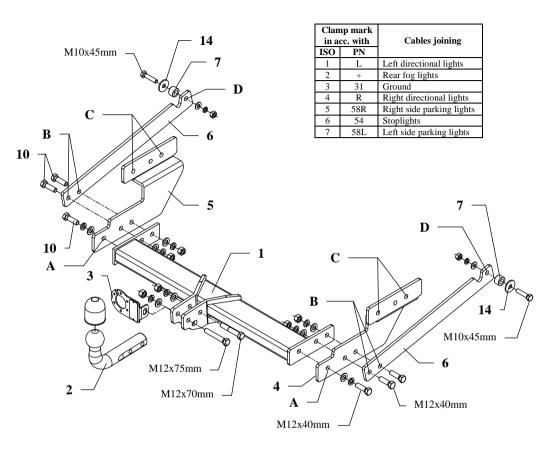
This towing hitch is designed to assembly in following cars: **VOLKSWAGEN T4 Transporter, Multivan, Caravelle, metal built-up, 2WD, 4WD,** produced since 01.1996 till 01.2003, catalogue no. **K27** and is prepared to tow trailers max total weight **2500 kg** and max vertical load **100 kg**.
