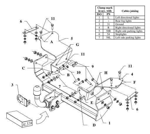
This towbar is designed to assembly in following cars: **ALFA ROMEO 147, 3/5 doors**, **except TI-Model, GTA3.2L 184KW** produced since 2000, catalogue no. **AL37A** and is prepared to tow trailers max total weight **1300 kg** and max vertical load **60 kg**.
