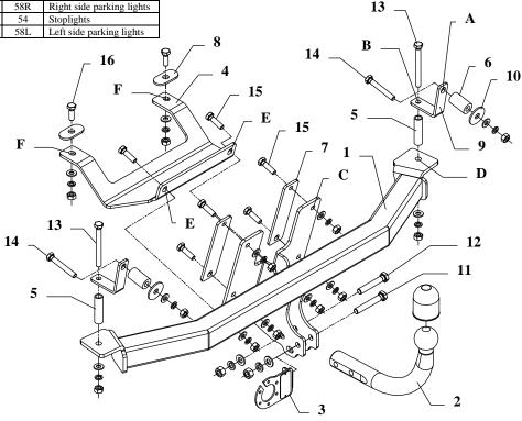
This towing hitch is designed to assembly in following car: **ALFA ROMEO 146, 5 doors,** produced since 1995 till 2001, catalogue no. **AL32** and is prepared to tow trailers max total weight **1300 kg** and max vertical load **75 kg**.
