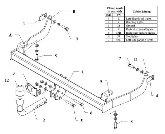
This towing hitch is designed to assembly in following cars: **VOLKSWAGEN CADDY**, **passenger car/delivery van**, produced since 11.1995 till 01.2004 and **SEAT INCA**, **passenger car/delivery van** produced since 11.1995 till 06.2003, catalogue no. **K31** and is prepared to tow trailers max total weight **1100kg** and max vertical load **50 kg**.
