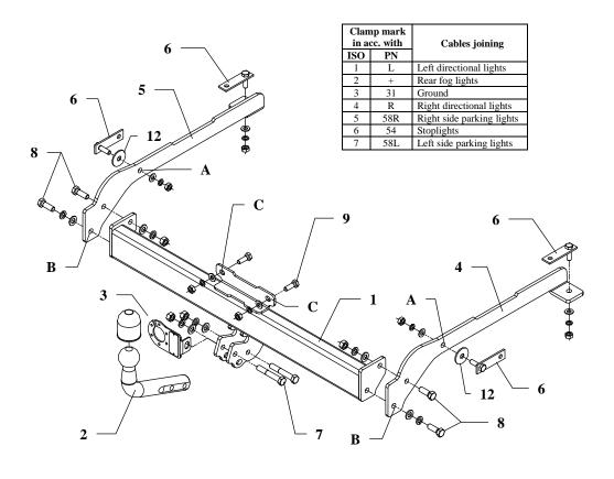
This towing hitch is designed to assembly in following cars: **PEUGEOT 605, 4 doors,** produced since 05.1990 till 09.1999, catalogue number **F10** and is prepared to tow trailers max total weight **1500 kg** and max vertical mass **75 kg**.
