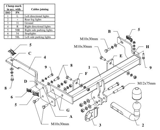
This towing hitch is designed to assembly in following cars: **PEUGEOT 106, 3/5 doors,** produced since 05.1996 till 07.2003, catalogue no. **F01** and is prepared to tow trailers max total weight **1100 kg** and max vertical load **50 kg**.
