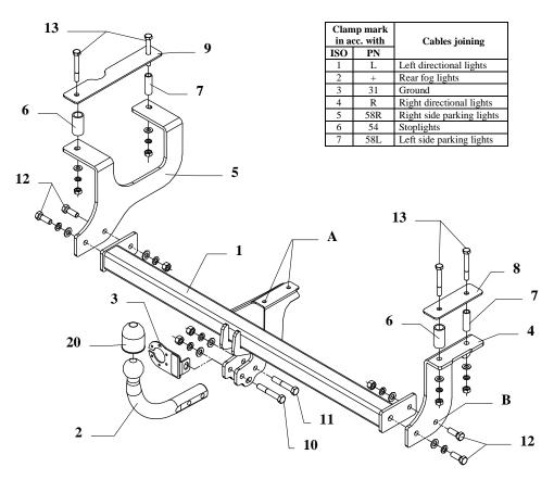
This towbar is designed to assembly in following cars: **SUZUKI WAGON R+, 5D** and **OPEL AGILA, 5D** produced since 04.2000 till 09.2002, catalogue no. **W14** and is prepared to tow trailers max total weight **1000 kg** and max vertical load **30 kg**.
