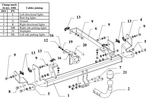
This towbar is designed to assembly in following cars: **Peugeot 807, Fiat Ulysse, Citroen C8, Lancia Phedra** (all 5 doors and VAN) produced since produced since 09.2002 till 10.2005 and since 11.2005 catalogue no. **F26** and is prepared to tow trailers max total weight **1850 kg** and max vertical load **76 kg**.
