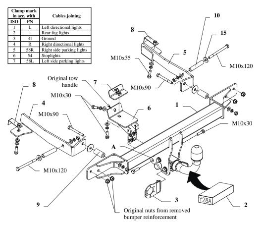
This towing hitch is designed to assembly in following cars: HONDA ACCORD TOURER Estate (CM1, CM2, CN2), except Type S and except 2,4L engine, produced since 05.2003 till 07.2008, catalogue no. Y28A and is prepared to tow trailers max total weight 1500 kg and max vertical load 75 kg.
