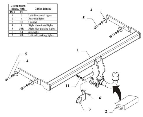
This towbar is designed to assembly in following car: **RENAULT MEGANE II, 4 doors,** produced since 09.2003 till 10.2012, catalogue no. **G43A** and is prepared to tow trailers max total weight **1300** kg and max vertical load **75kg**.
