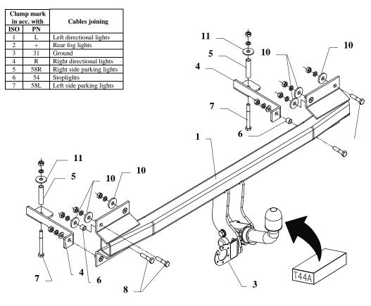
This towing hitch is designed to assembly in following car: **KIA SEPHIA 4/5 door (FA),** produced since 01.1995 till 05.1998, catalogue no. **T44A** and is prepared to tow trailers max total weight **1450** kg and max vertical load **50 kg**.
