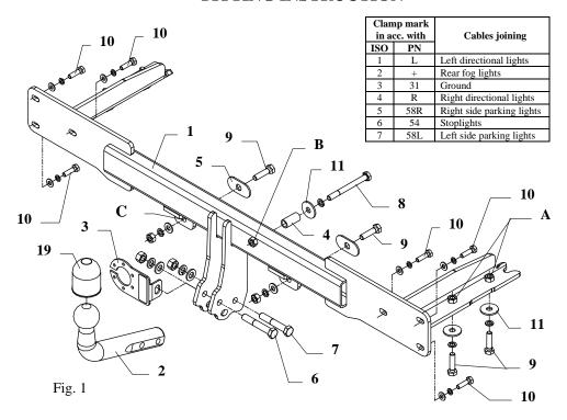
This towing hitch is designed to assembly in following cars: **KIA CARNIVAL (UP) VAN**, produced since 1997 till 04.1999, catalogue no. **T14** and is prepared to tow trailers max total weight up to **2000 kg** and max vertical load **80 kg**.
