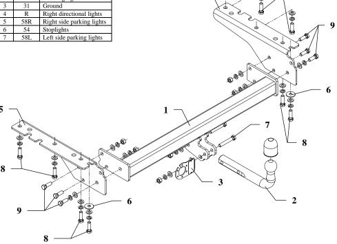
This towing hitch is designed to assembly in following cars: JEEP CHEROKEE (XJ/J), produced since 04.1997 till 08.2001, catalogue no. JP01 and is prepared to tow trailers max total weight up to 3300 kg and max vertical load 100 kg.
