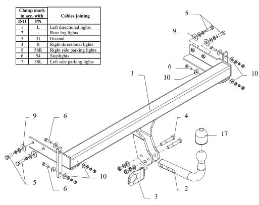
This towbar is designed to assembly in following cars: **HYUNDAI SONATA, 4 doors (EM, EF),** produced since 06.2001 till 02.2005, catalogue no. **J50** and is prepared to tow trailers max total weight **1700 kg** and max vertical load **75 kg**.
