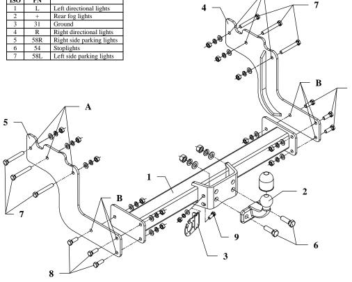
This towing hitch is designed to assembly in following cars: FORD TRANSIT ER, lengthened frame, loading platform, produced since 11.1991 till 04.2000, catalogue no. C21 and is prepared to tow trailers max total weight 2000 kg and max vertical mass 75 kg.
