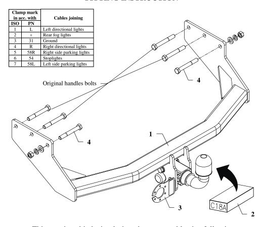
This towing hitch is designed to assembly in following cars: **FORD TRANSIT, metal build-up, also MAXI, loading platform,** produced since 11.1991 till 04.2000, catalogue no. **C18A** and is prepared to tow trailers max total weight **2000 kg** and max vertical mass **75 kg**. Towbar is designed in way excluding diassemble, cut out or drill a bumper.
