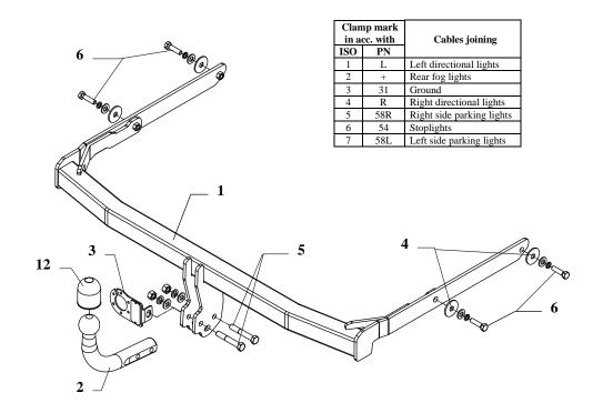
This towing hitch is designed to assembly in following car: **FORD FUSION, 5 doors, VAN,** produced since 09.2002 till 09.2005 and since 10.2005, catalogue no. **C43** and is prepared to tow trailers max total weight **900 kg** and max vertical load **50 kg**.
