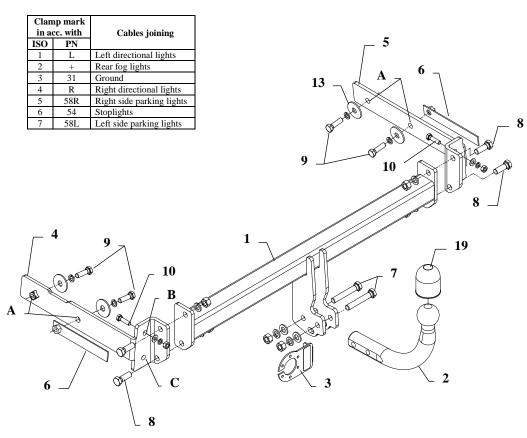
This towbar is designed to assembly in following cars: **FORD FOCUS I, 4 doors (Mk1), except RS**, produced since 01.1999 till 04.2005, catalogue no. **C28** and is prepared to tow trailers max total weight **1635 kg** and max vertical load **50 kg**.
