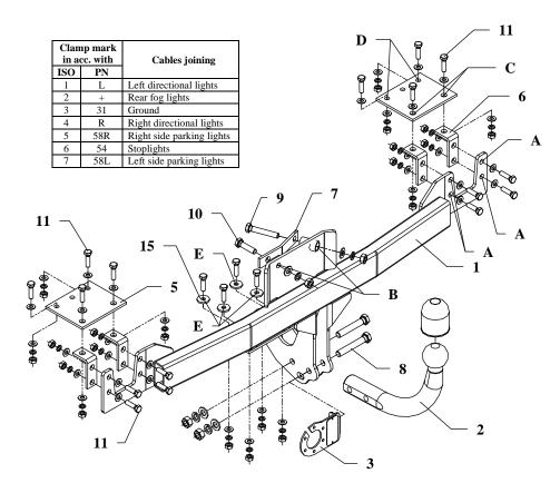
This towing hitch is designed to assembly in following car: **FIAT BRAVO, 3 doors (182),** produced since 09.1995 till 10.2001, catalogue no. **R10** and is prepared to tow trailers max total weight **1400 kg** and max vertical load **75 kg**.
