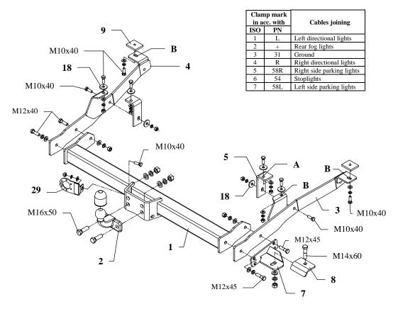
This towing hitch is designed to assembly in following cars: **FIAT DUCATO II, metal build-up, loading platform, 4x4, PEUGEOT BOXER, metal build-up, loading platform, CITROEN JUMPER, metal build-up, loading platform,** produced since 07.1999 till 05.2006, catalogue number **R24** and is prepared to tow trailers max total weight **2000 kg** and max vertical load **100 kg**.
