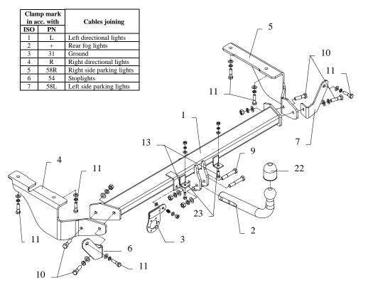
This towbar is designed to assembly in following cars: **CITROEN C5 I Break, ESTATE,** produced since 10.2004 till 03.2008, catalogue no. **P30** and is prepared to tow trailers max total weight **1600 kg** and max vertical load **85 kg**.
