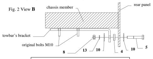
Torque settings for nuts and bolts (8,8): **M 8 -** 25 Nm **M 10 -** 55 Nm
