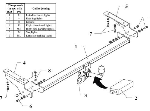
This towbar is designed to assembly in following cars: CITROEN C5 I, 4/5 doors, (X41), produced since 04.2001 till 09.2004, catalogue no. P24A and is prepared to tow trailers max total weight 1600 kg and max vertical mass 85 kg.
