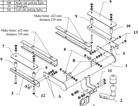
This towbar is designed to assembly in following car: CITROEN SAXO 3/5 doors, produced since 05.1996 till 09.2003, catalogue no. P09 and is prepared to tow trailers max total weight 1100kg and max vertical load 50 kg.
