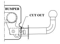
4. To the chassis of car put main bar of the towbar (pos. A) and through holes pos. 2 and 3 fix with already mounted side brackets (pos. C) using bolts M10x45mm.
