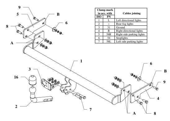
This towbar is designed to assembly in following car: CITROEN ZX 3/5 DOORS (N2), produced since 03.1991 till 06.1997, catalogue number P 03, and is prepared to tow trailers max total weight 1100 kg and max vertical load 70 kg.
