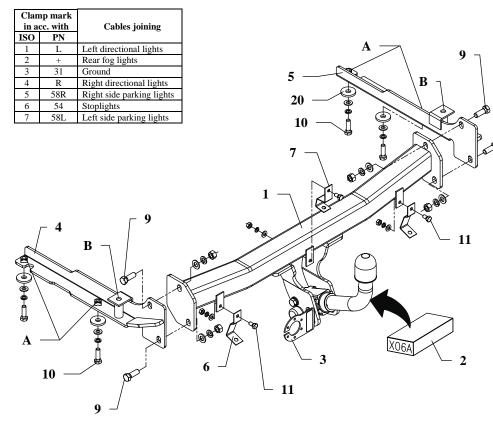
This towing hitch is designed to assembly in following cars: **DAEWOO NUBIRA, 4 door (100),** produced since 06.1997 till 06.1999, catalogue no. **X06A** and is prepared to tow trailers max total weight **1200 kg** and max vertical load **70 kg**.
