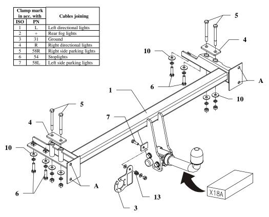
This towbar is designed to assembly in following cars: CHEVROLET LACETTI ESTATE, produced since 2005, catalogue no. X18A and is prepared to tow trailers max total weight 1200 kg and max vertical load 75 kg.
