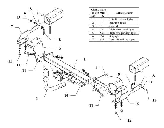
This towing hitch is designed to assembly in following cars: **TOYOTA YARIS, 3/5 doors, (CP10), Japanese and French version except TS,** produced since 04.1999 till 12.2005, catalogue no. **O24** and is prepared to tow trailers max total weight **900 kg** and max vertical load **50 kg**.
