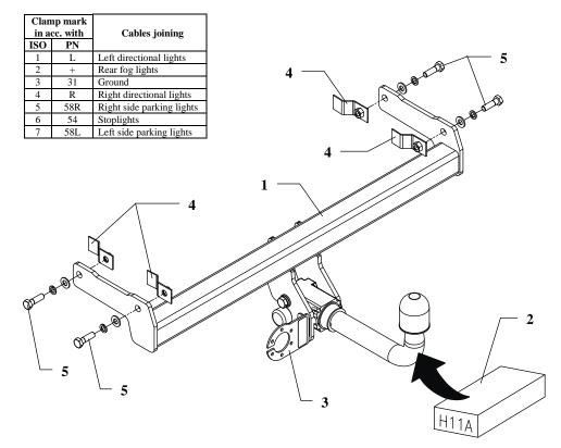
This towing hitch is designed to assembly in following cars: SKODA FELICIA, PICK-UP, produced since 02.1996 and VOLKSWAGEN CADDY, PICK-UP, produced since 06.1996 till 12.2000, catalogue no. H11A and is prepared to tow trailers max total weight 1000 kg and max vertical mass 50 kg.
