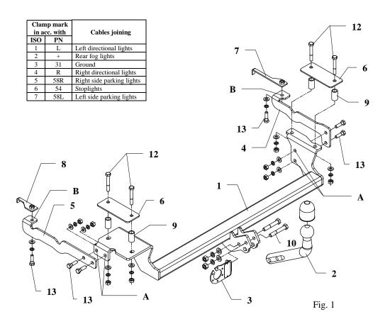
This towing hitch is designed to assembly in following cars: **SEAT CORDOBA**, **2/4 doors**, produced since 02.1993 till 01.1996, catalogue no. **SC40** and is prepared to tow trailers max total weight **1200 kg** and max vertical load **50 kg**.
