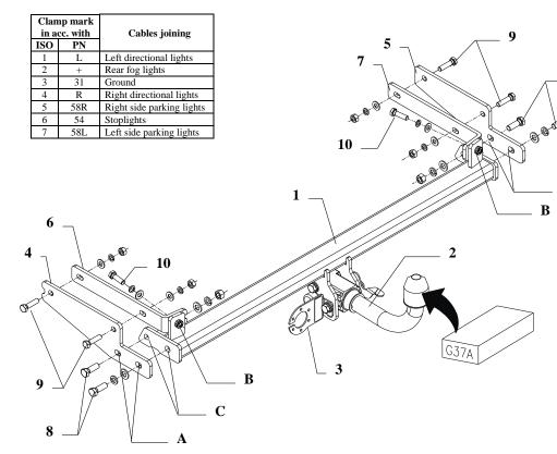
This towing hitch is designed to assembly in following cars: **RENAULT THALIA, 4 doors,** produced since 06.2001 till 08.2008 and since 09.2008, catalogue no. **G37A** and is prepared to tow trailers max total weight **1150 kg** and max vertical load **75 kg**.
