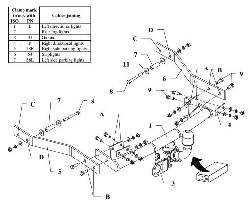
This towing hitch is designed to assembly in following cars: **RENAULT 19, 3/5 doors** and **4 doors, cabrio,** produced since 05.1988 till 05.1995, catalogue no. **G05A** and is prepared to tow trailers max total weight **1200 kg** and max vertical mass **75 kg**.
