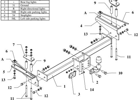
This towbar is designed to assembly in following cars: NISSAN PATROL GR, 3/5 DOORS (Y60), produced since 08.1987 till 12.1997, catalogue no. V09 and is prepared to tow trailers max total weight 3000 kg and max vertical load 100 kg.
