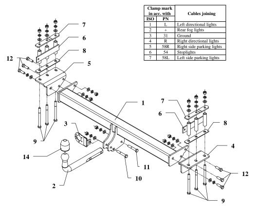
This towbar is designed to assembly in following cars: **NISSAN PATROL 3/5 door (Y61),** produced since 01.1998 till 09.2004, catalogue no. **V02** and is prepared to tow trailers max total weight up to **3500 kg** and max vertical mass **140 kg**.
