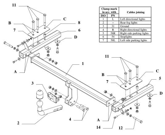
This towbar is designed to assembly in following cars: **KIA CARENS I II**, (FC, FJ) VAN, produced since 01.2000 till 08.2006, catalogue no. **T43** and is prepared to tow trailers max total weight **1250 kg** and max vertical load **75 kg**.
