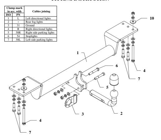
This towing hitch is designed to assembly in following cars: **MITSUBISHI PAJERO**, **V20**, **(V2/V4)**, **3/5 doors**, produced since 12.1990 till 05.2000, catalogue no. **Z02** and is prepared to tow trailers max total weight **3300 kg** and max vertical mass **135 kg**.
