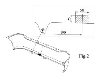
9. Complete paint layer damaged during installation.
