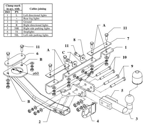
This towbar is designed to assembly in following cars: **SKODA FAVORIT, 5 doors,** produced since 05.1989 till 08.1994, catalogue no. **H03** and is prepared to tow trailers max total weight **900 kg** and max vertical load **50 kg**.
