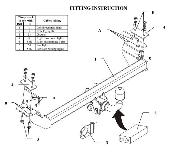
This towbar is designed to assembly in following cars: **TOYOTA COROLLA Station Wagon KOMBI (E11)** produced since 06.1997 till 12.2001, catalogue no. **O17A** and is prepared to tow trailers max total weight **1400 kg** and max vertical load **75 kg**.
