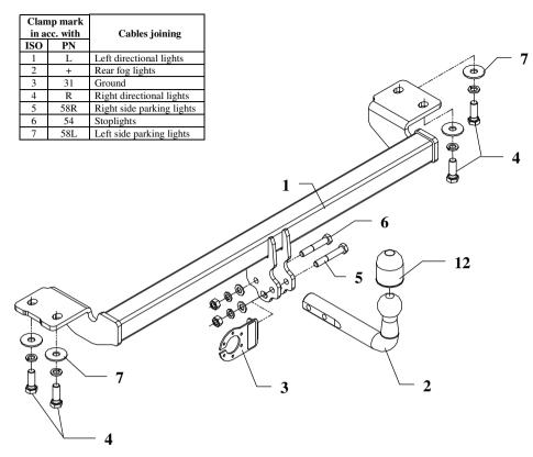
This towbar is designed to assembly in following cars: **TOYOTA AVENSIS ESTATE**, produced since 02.1998 till 03.2003, catalogue no. **O20** and is prepared to tow trailers max total weight **1575 kg** and max vertical mass **75 kg**.
