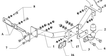
This towing hitch is designed to assembly in following car: **FORD TRANSIT CONNECT** produced since 2002 till 12.2012, catalogue no. **C46** and is prepared to tow trailers max total weight up to **1200 kg** and max vertical load **75 kg**.
