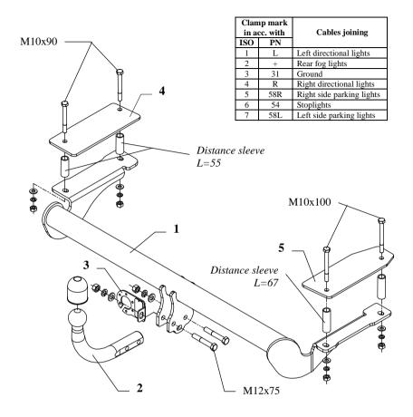
This towbar is designed to assembly in following cars: **OPEL ASTRA "G" 4 door**, produced since 10.1998 and **OPEL ASTRA** "G" 3/5 door, produced since 03.1998, catalogue no. **E21** and is prepared to tow trailers max total weight **1500 kg** and max vertical load **75 kg**.
