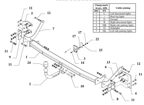
This towbar is designed to assembly in following car: **PEUGEOT 407 4 door,** produced since 2004 till 08.2008 (**Attention! Not suitable for car with 3.0 HDi V6 engine!**), catalogue number **F29** and is prepared to tow trailers max total weight **1900 kg** and max vertical load **65 kg**.
