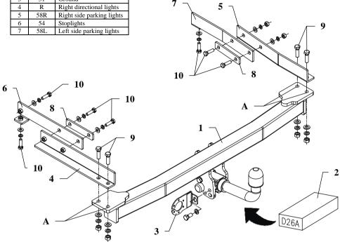
This towbar is designed to assembly in following cars: **MERCEDES S CLASS (W140)**, produced since 1991 till 1999, catalogue no. **D26A** and is prepared to tow trailers max total weight **2000 kg** and max vertical mass **75 kg**.
