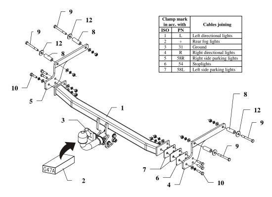
This towbar is designed to assembly in following car: **DACIA LOGAN, 4 doors,** produced since 09.2004 till 12.2012, catalogue number **G47A** and is prepared to tow trailers max total weight **1100 kg** and max vertical load **75 kg**.
