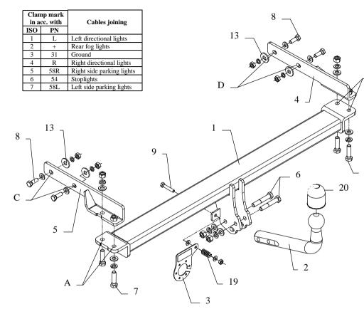
This towing hitch is designed to assembly in following cars: MERCEDES S210 CLASS E, ESTATE, produced since 1996 till 03.2002, catalogue no. D31 and is prepared to tow trailers max total weight 2300 kg and max vertical load 90 kg.
