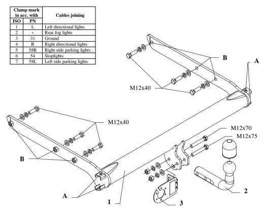
This towbar is designed to assembly in following cars: **VOLKSWAGEN T4 TRANSPORTER**, **4x4**, **2x4**, produced since 08.1990 till 01.1996, catalogue no. K12 and is prepared to tow trailers max total weight **2500 kg** and max vertical mass **100 kg**.
